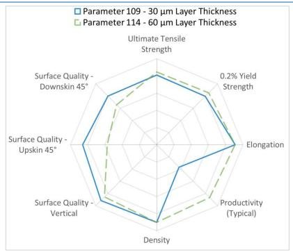
Spider Plot is generated by normalizing typical material data (containing both horizontal and vertical data) against a range defined for each material family. For **Titanium Alloys**, the ranges are as follows: UTS: 0-1200 MPa, 0.2%YS: 0-1100 MPa, Elongation: 0-20%, Density: 99-100%, Productivity: 5-30 cm<sup>3</sup>/hr, Surface Quality (all): 50-4 µm
