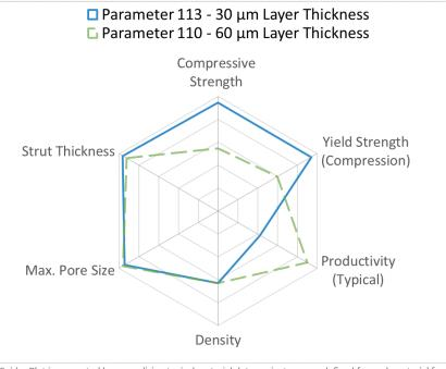
Spider Plot is generated by normalizing typical material data against a range defined for each material family. For **Titanium Alloys (mesh parameter)**, the ranges are as follows: UTS 0-110 MPa, 0.2%YS: 0-85 MPa, Density: 0-100%, Productivity: 5-40 cm<sup>3</sup>/hr, Max. Pore Size: 0-510 μm, Strut Thickness: 0-260 μm
